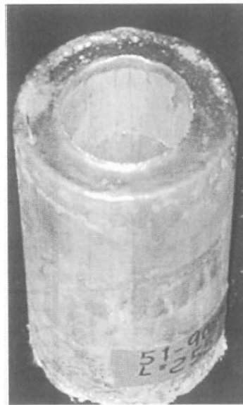
Fig.11 Oblique Top View of Hollow Ingot
